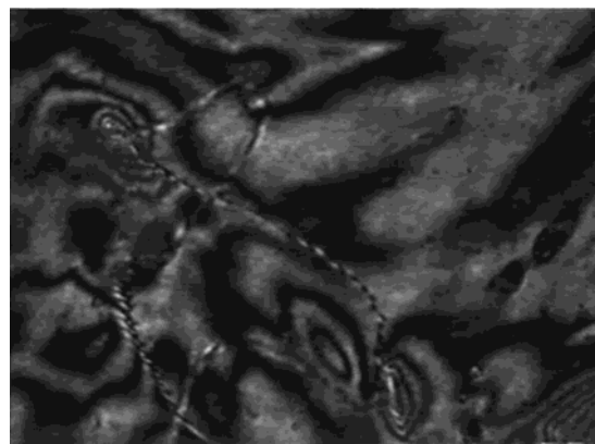
Figure 5. Micrograph of nonplanar loops viewed between crossed polars, oriented at 45^\circ to the preferred orientation (the extrusion direction), which is along the diagonal of the image. Conditions: PPTA; L_w = 235 \mu\text{m} ; w = 0.105 ; 400 \mu\text{m} thick cell.
